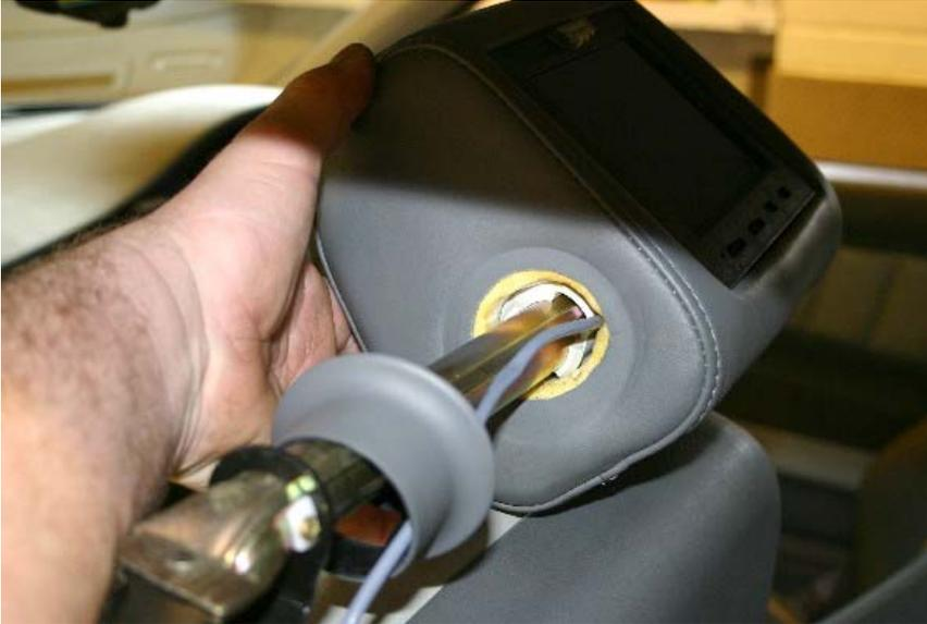
15. Refit the headrest front shell with the #10 Torx screws.
