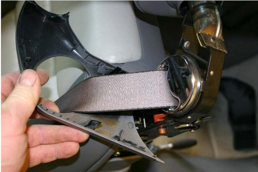
7. Remove the plastic screw cover to reveal the #20 Torx screw at the bottom of the seat and remove the screw.
