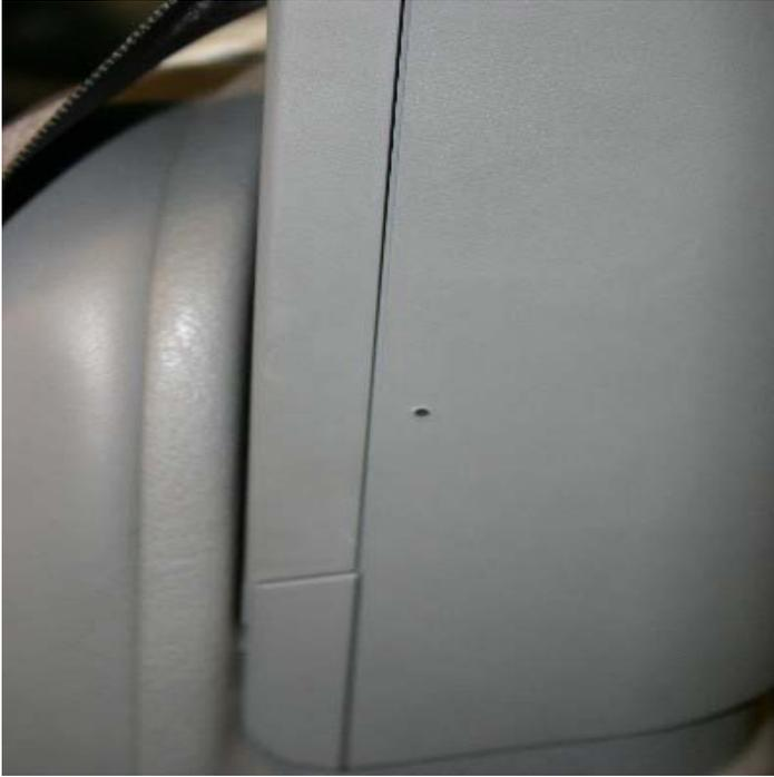
3. This then releases the arm rear shell. Disregard the blue cable in the picture. It is for the Headrest monitor.
