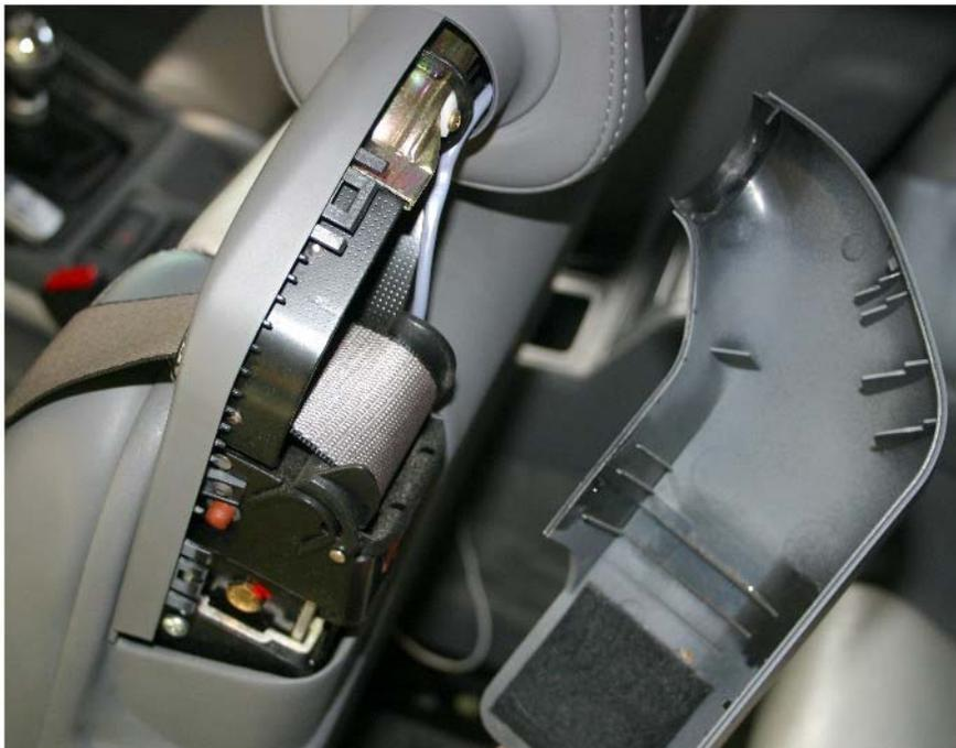
4. The headrest is held on a nylon friction sleeve. Whilst gently rotating the headrest forwards and back, slide the headrest away about 3 inches.
