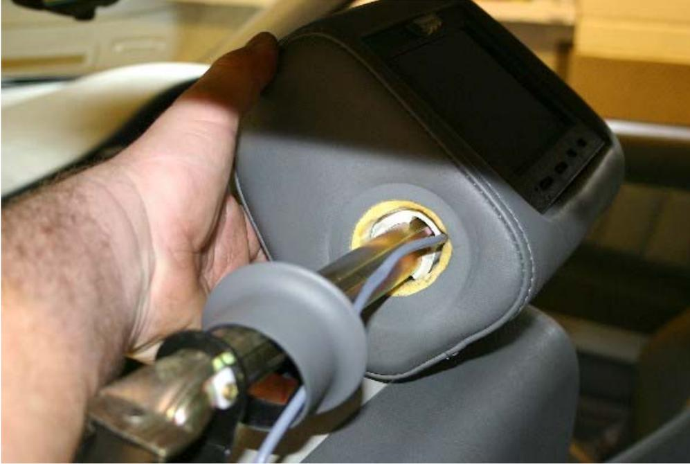
5. Lower the seat fully, which will raise the headrest fully to allow access to the 2 (1 on each side), #10 Torx screws which retain the arm front shell.
