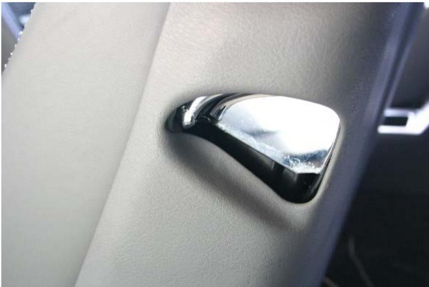
2. Now move the headrest a little by pushing it away while rotating. To move the headrest arm rear shell, push the straightened paper clip into this hole in the head rest arm shell to release the clips. Please note that on newer E31s there are 2 of these holes and releases. 1 on each side of the headrest arm.
