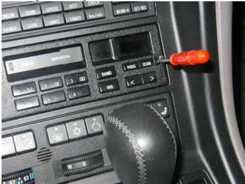
Insert your small screwdriver and unscrew until you feel resistance. Then with a couple of fingers inside the cassette slot, pull the radio out of the dash.
