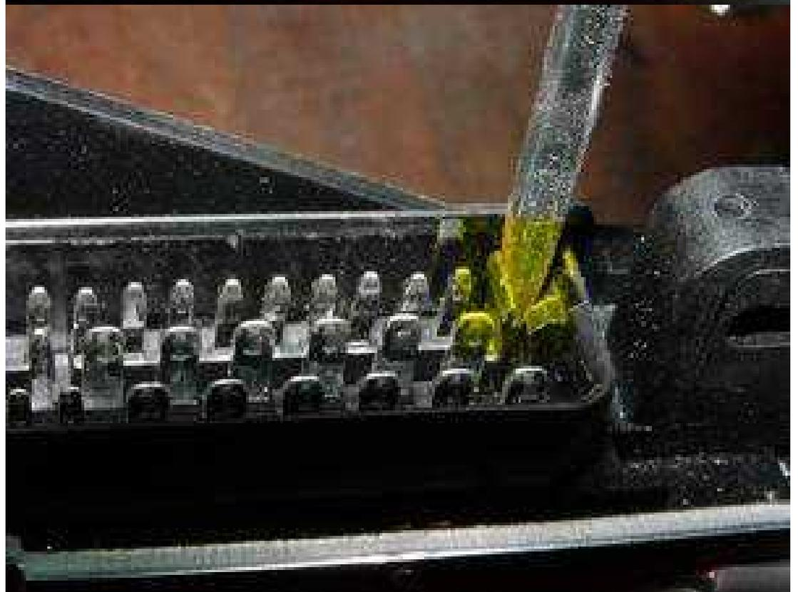
Now the horizontal clamping needs to be opened, which is tricky but possible...
