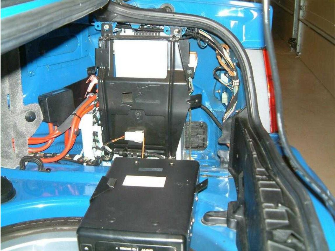
Next, you must remove the mounting bracket. It is secured by four 10mm nuts, two at the top, and two at the bottom. Once the nuts are removed, you can lay the bracket down flat in the trunk. The Euro CSI has the AHK control unit mounted on the back side of the CD mounting bracket, and it is visible in the following photo:
