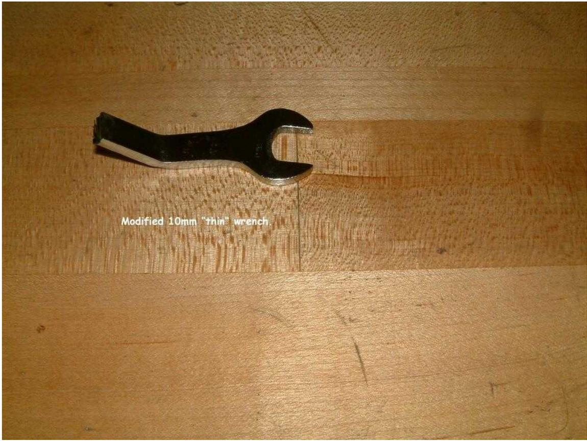
Actually holding the 10mm nut in place with my "special" tool also required some thought. I finally realized the nut could be held to the wrench by using some masking tape on the bottom of the nut that also wrapped onto the wrench.
