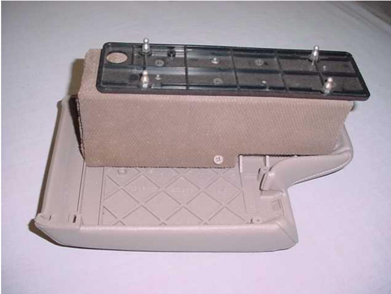
This is the Arm Rest after I screwed it to the wooden block and plastic part. Note: the four medal pins, they will snap into the medal frame located inside the console.
