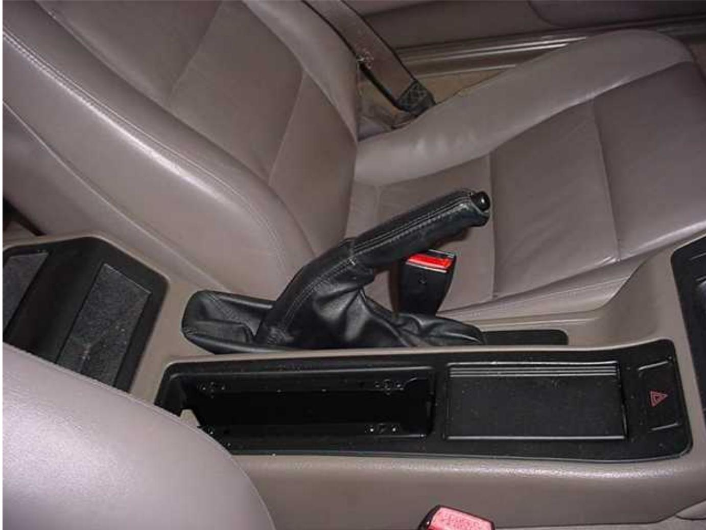
This is what the console looks like after the Phone has been removed. There is a metal frame that fits inside and a plastic piece that the Phone is attached to. I left the metal frame bolted inside and kept the plastic piece to screw the Arm Rest too.
