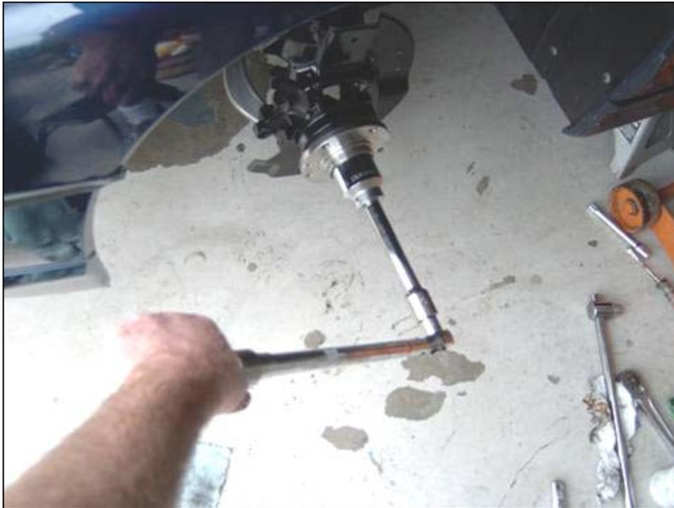
Figure 11 - Torqueing the Hub Nut
