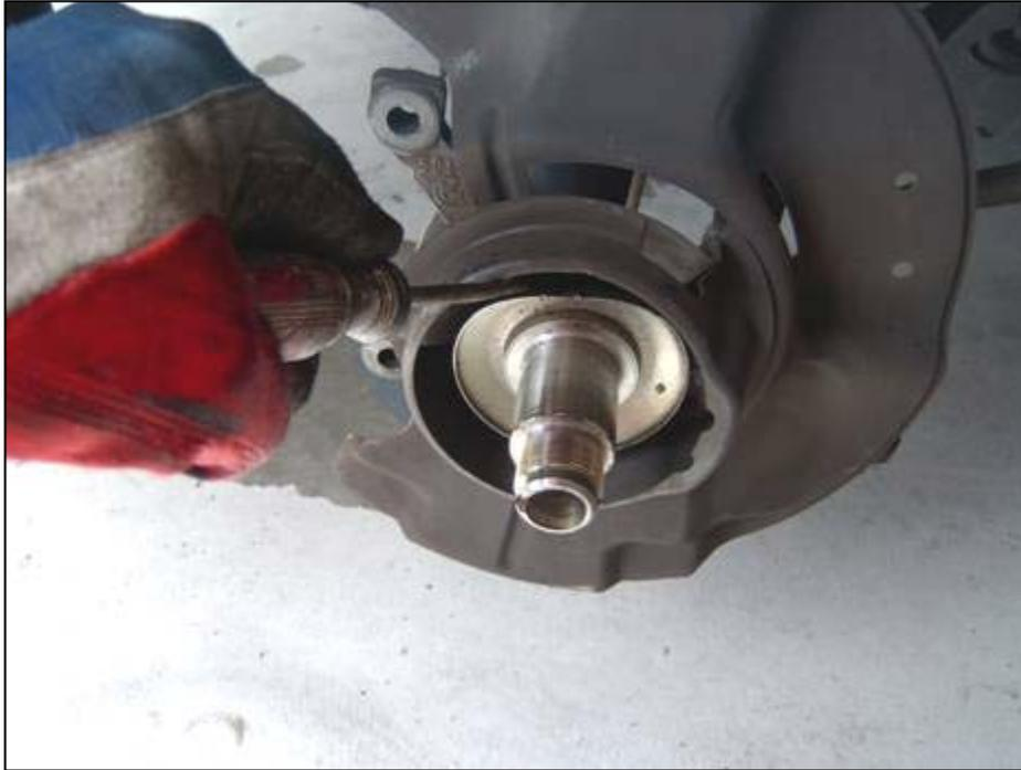
**Figure 7 - Removing the Dust Collar**
