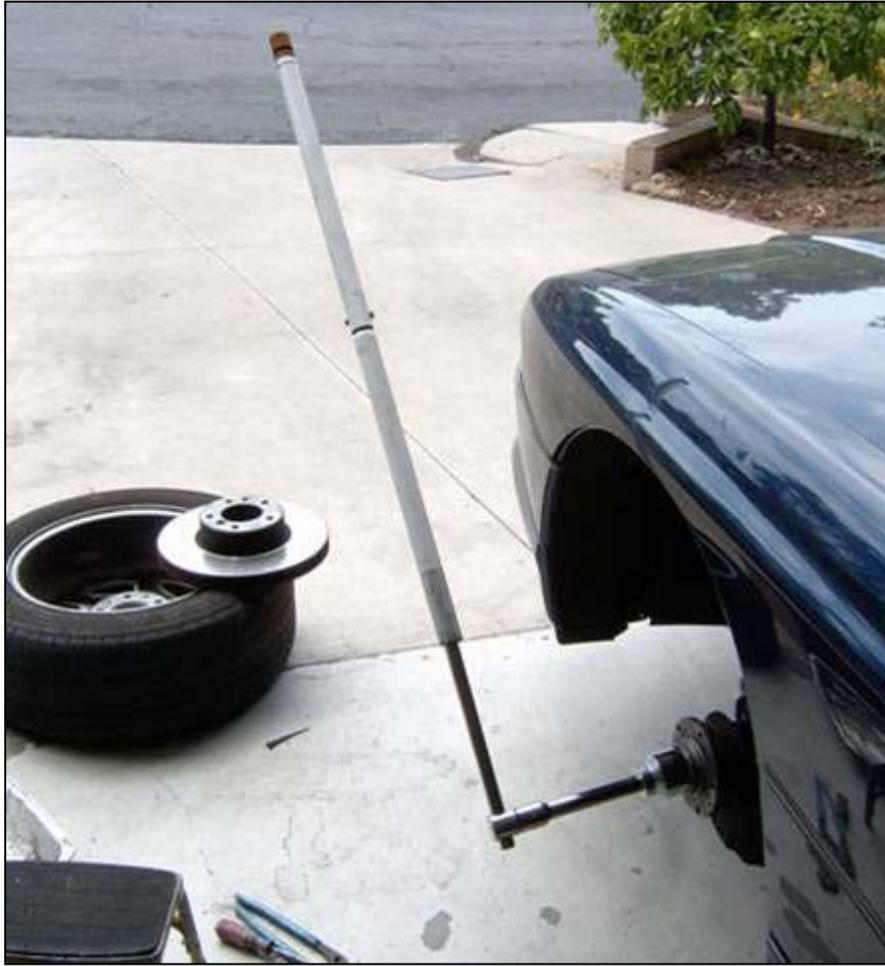
Figure 6 - Removing the Hub Nut
