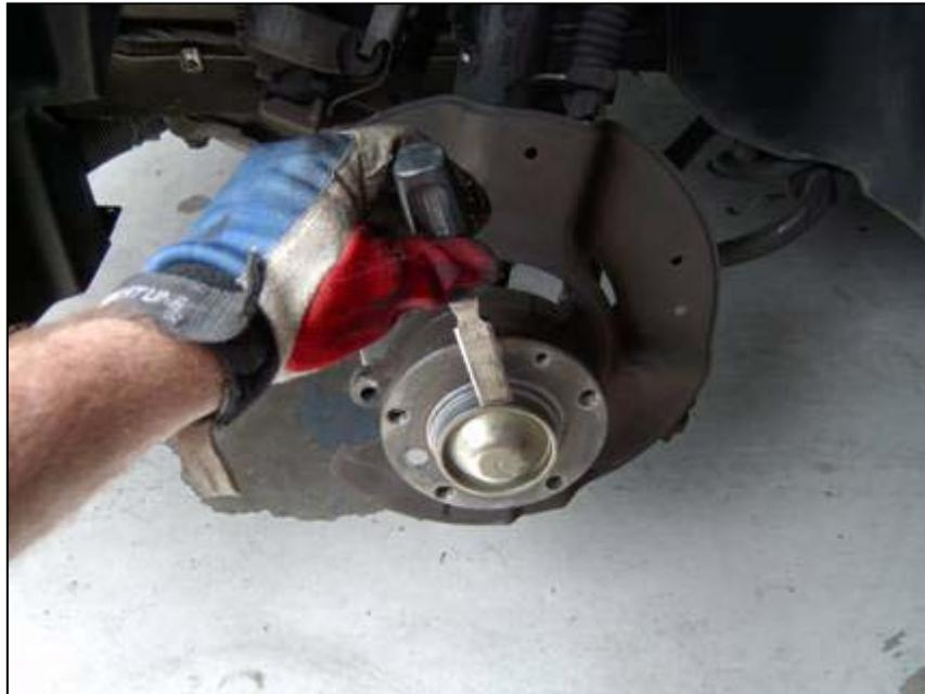
**Figure 4 - Removing the Grease Cap**
