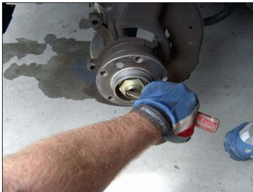
**Figure 5 - Unstaking the Hub Nut**
