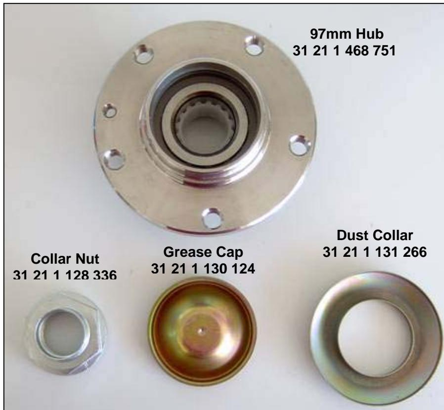
**Figure 1 - E31 Front Hub/Bearing Assembly**
