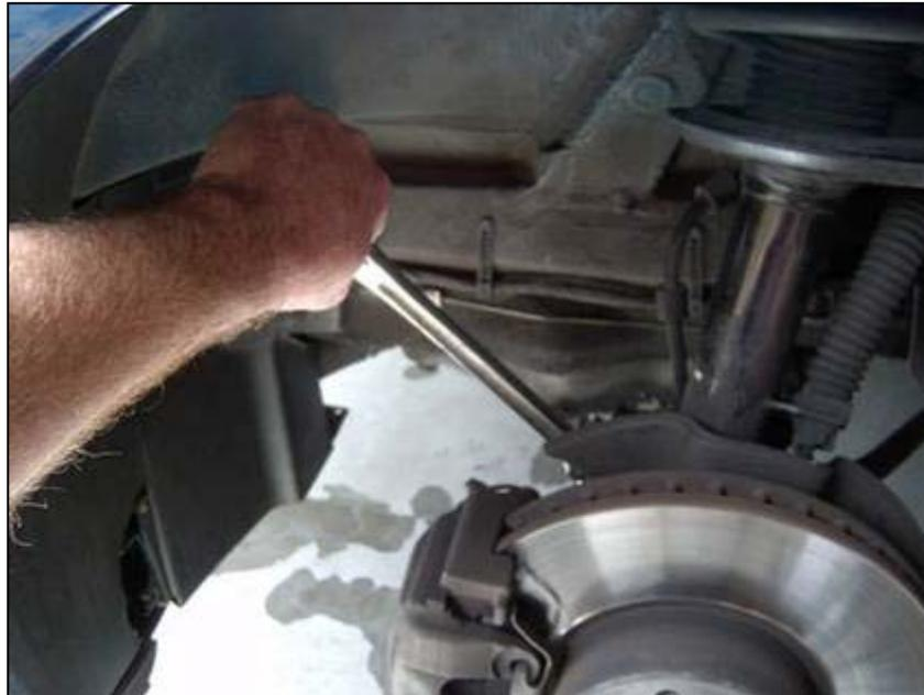
Figure 3 - Removing the Caliper
