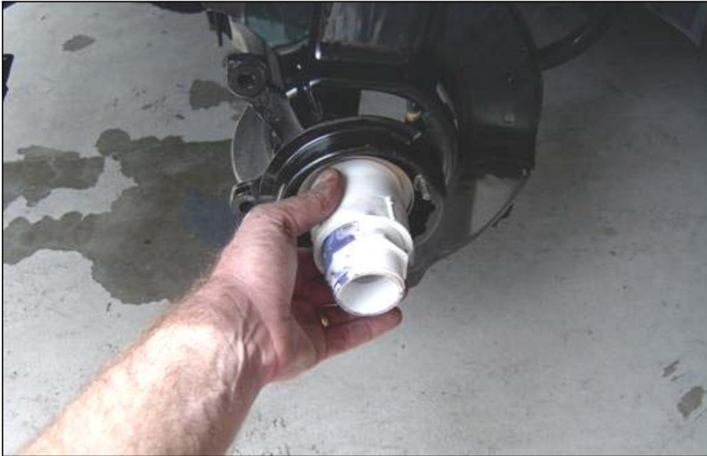
Figure 9 - Installing the Dust Collar
