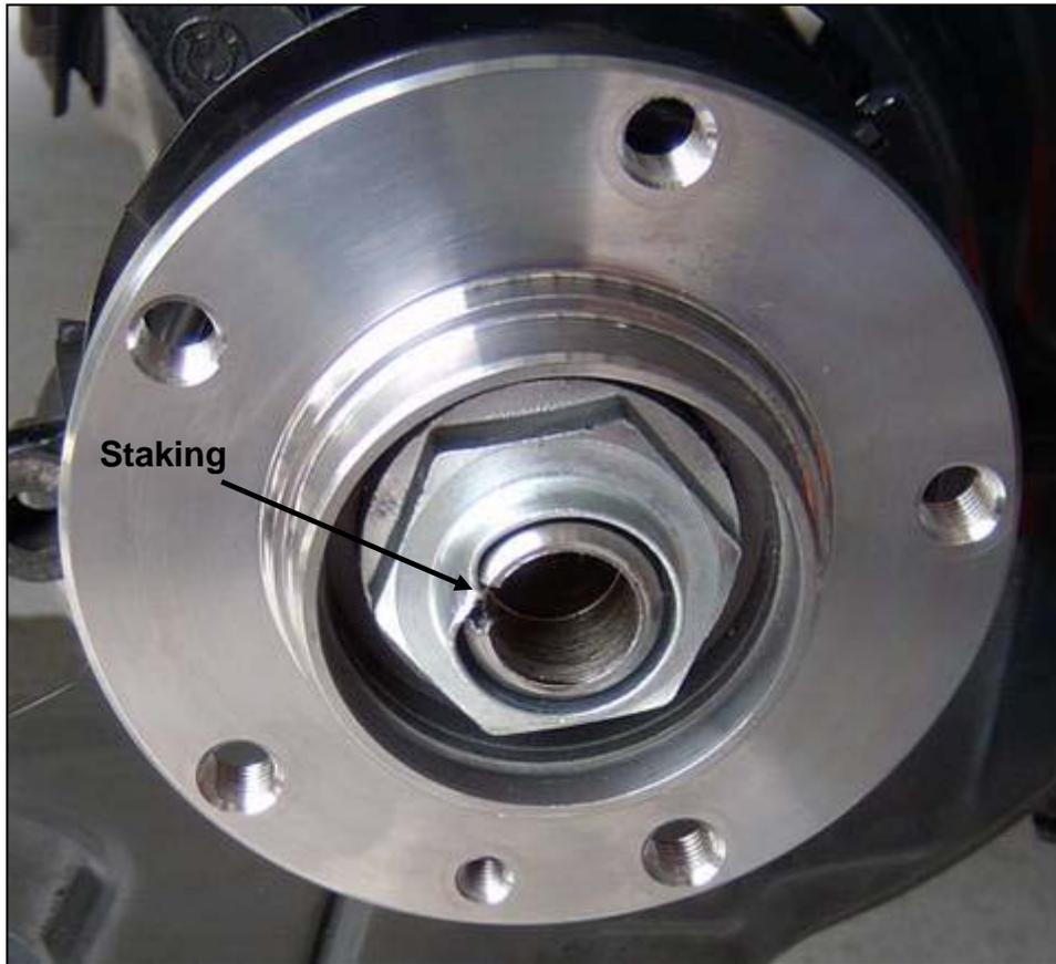
**Figure 12 - Staking the Hub**
